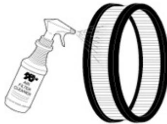
Spray K&N air filter cleaner liberally onto the entire element and let soak for 10 minutes.
