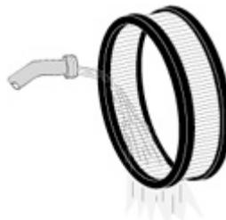
Rinse off the element with low water pressure, tap water is OK. Always flush from the clean side to dirty side. This removes the dirt and does not drive it into the filter.
