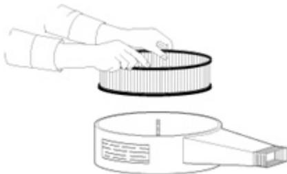
Re-install your K&N air filter element with proper care. Make sure the element seats properly in the filter case. Install the cover making sure it's in the right position. Tighten all the nuts, bolts, screws or clips to factory specifications.
